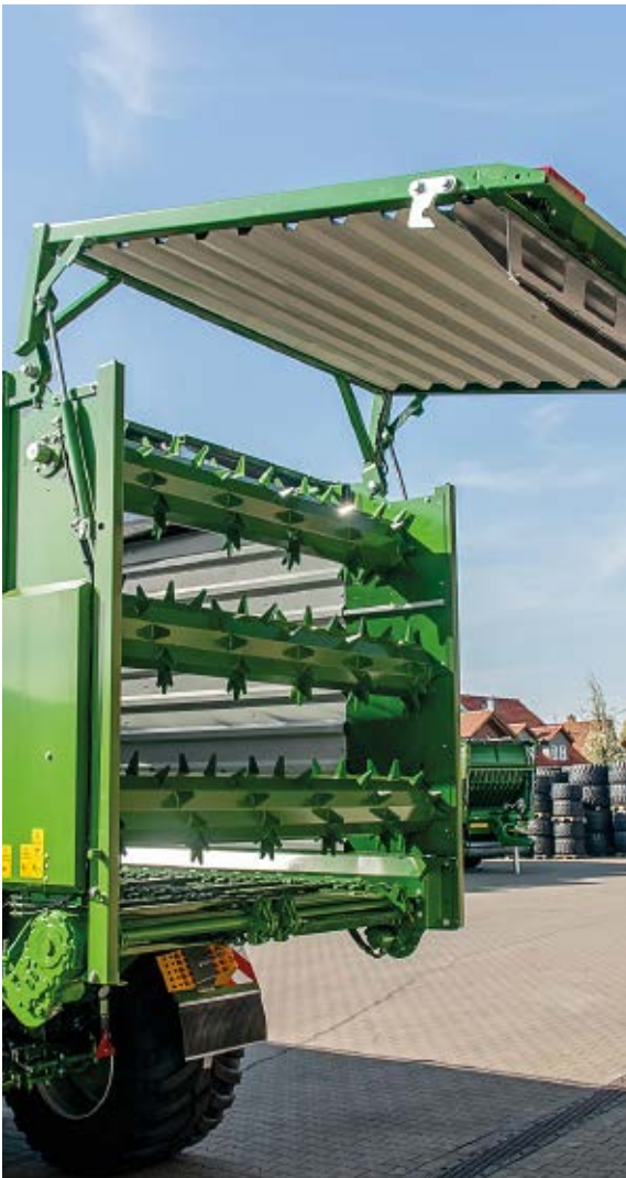
Wide opening, sturdy tailgate with mechanical locking – for fast unloading.
