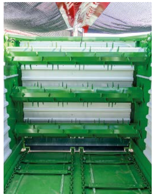
The S-model dosing unit with three standard dosing rollers (SHUTTLE 450 S / SHUTTLE 490 S).
