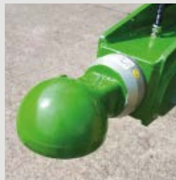
Drawbar eye with measuring device
