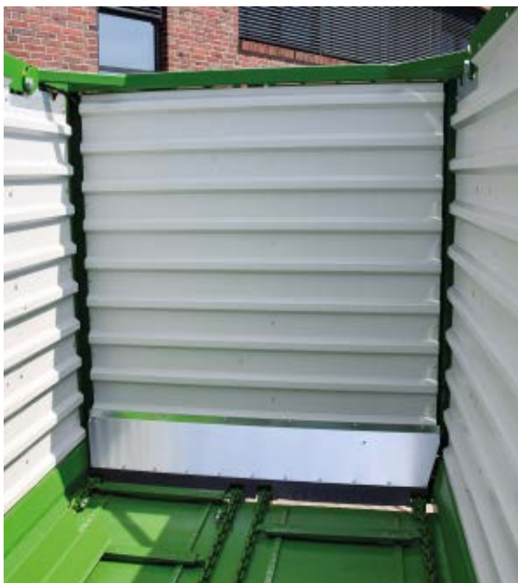
K-model without dosing rollers (SHUTTLE 470 K / SHUTTLE 510 K)
